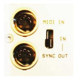
At the Sync socket there is a Sync Out signal that can be used to synchronise other gear with Sync In.
