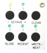
The LEDs over the keys indicate the programming of Octave Up/Down, Slide, Accent, of the note.
