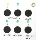
Then a new Pattern can be selected. Press the Write/Next buttom, and the second Pattern is fixed in the TRACK. The selected Pattern is sequentially repeated as in the Pattern Play mode. As in the Pattern Play mode you can chain several Pattern and be written with a Write/Next completely in the track.
