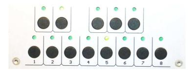
The active pattern is indicated with a flashing LED over the button. When pressing a new pattern, this LED lights continuously. After the pattern changed after the last step, to selected pattern, this LED flashes again.
