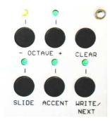
The LEDs over the buttons indicate the programming of Slide, Accent, Oktave Up/Down on the active note.
