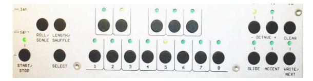
With pressing one of the buttoms 1-8 of the keyboard, the step is directly selected e.g. the step 7. Now this step can be changed.
