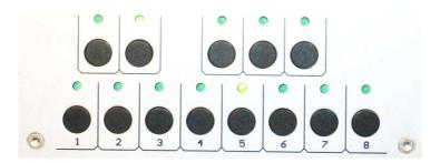
The active pattern is indicated with the LED over the buttom and is played repetitive. Press Write/Next and the current pattern becomes the first pattern of the track.
