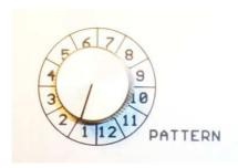
The pattern is selected from one of the 12 pattern groups. You can change the pattern group at all times with the rotary switch, and the switching into the new pattern group takes place after the last step of the current pattern.
