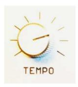
With Tempo, the speed of the internal clock generator is controlled. Start and stop with the Start/Stop buttom.
