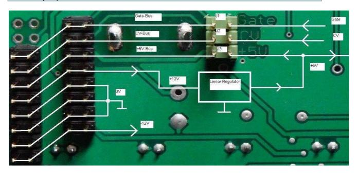
The +5V supply of the Autobot can be loaded up to 200mA.
