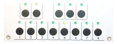
LEDs 1-4 of the step buttons will now indicate the shuffle setting of the first kind of shuffle.
