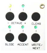
Press the buttom Write/Next again, and the step 3 is shown, etc.. After the last step of the patterns (dependent on the pattern length programming) the cursor jumps back on step 1.
