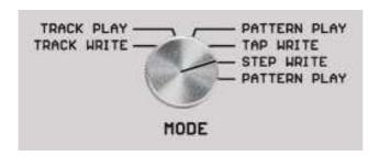
In this mode, unlike as in Pattern Tap Write Mode, you can only playback and edit a single pattern. The pattern to be edited depends on the pattern playing at the moment the mode is changed. This pattern will continue to play when the mode is switched back.
