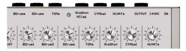
Output is for the mixed signal (6.3mm mono) of the instruments. Instruments connected by their individual out will not be present at the mix out. The volume of the mix out can be controlled with the Volume knob
