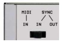
A Sync-out Signal will be generated at the Sync socket for other devices that have a Sync-In socket.
