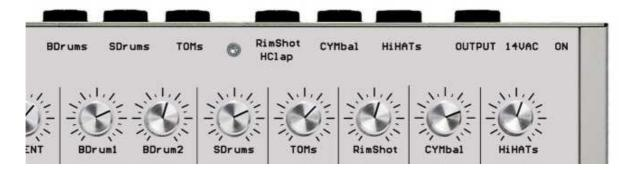
The sound circuitry of the Drumatix is mostly identical with the 606 and has been realized using present-day components. The sounds get many new parameters and new sounds are added.
