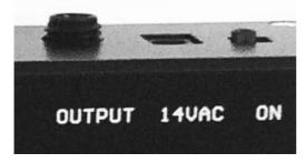
The Miami has an On/Off slide switch on the right side of the rear panel. Replacement AC Adapters can be ordered from acidlab.de.
