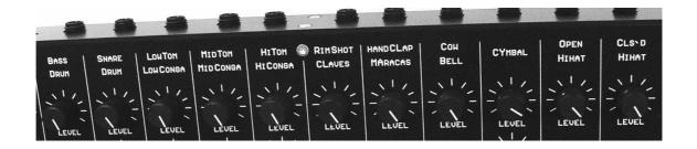
The sound circuitry of the Miami is identical with the 808 and has been realized using present-day components. Its sounds closely match the original 808.
