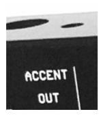
The Accent Out is primarily intended to be used to control an analog synthesizer with a gate input.
