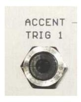
The Accent-/Trig1 Out is primarily intended to be used to control a Trigger- or Accent In of any drum-module or gate-/trigger input of an analog synthesizer, or any other event in your modular system.
