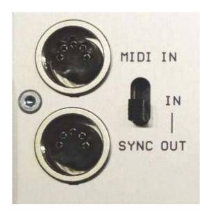
A Sync-out Signal will be generated at the Sync socket for other devices that have a Sync-In socket.
